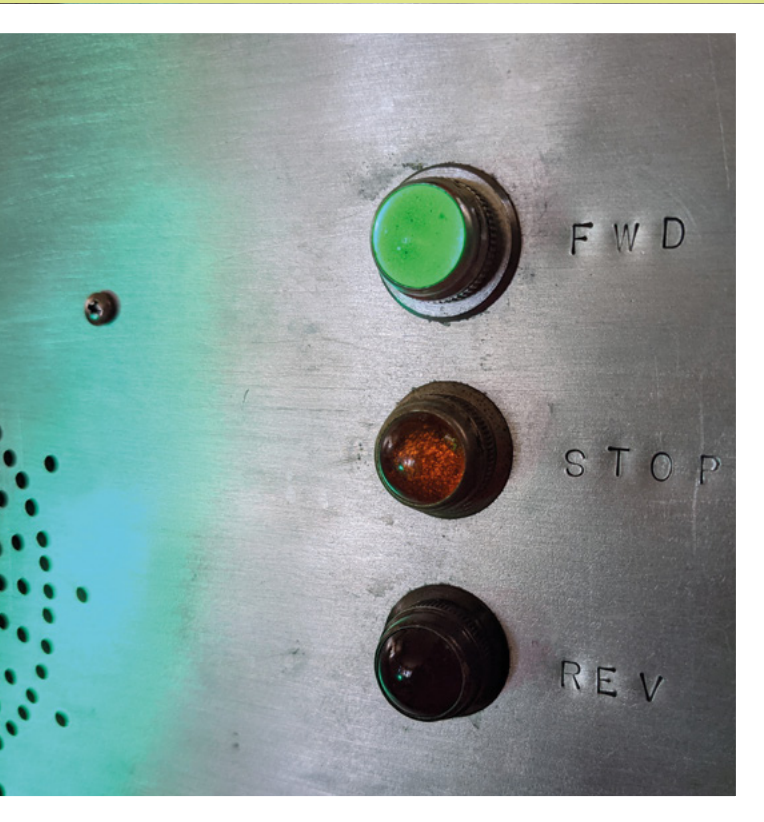
Left ♦ Panel mount LEDs make great retro-looking indicators
