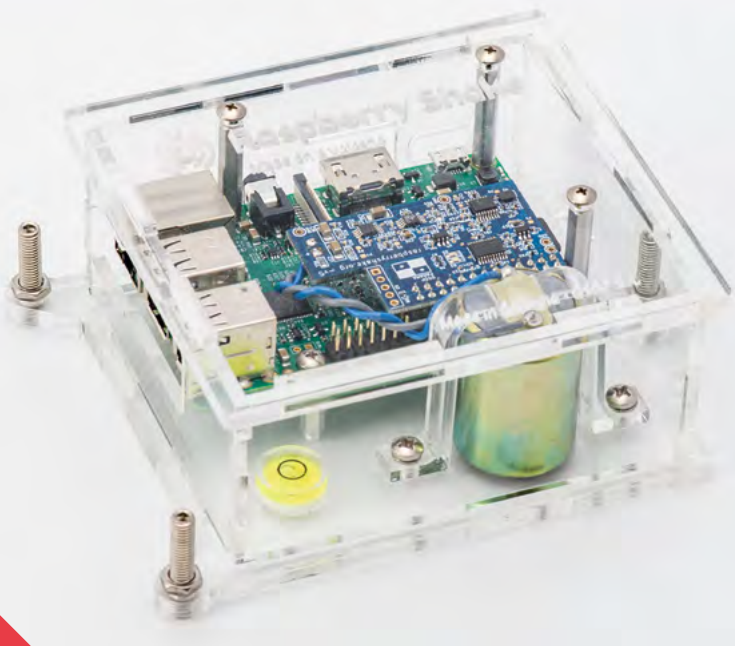
Above ♦ The standard RS1D Shake in its enclosure with a Raspberry Pi
