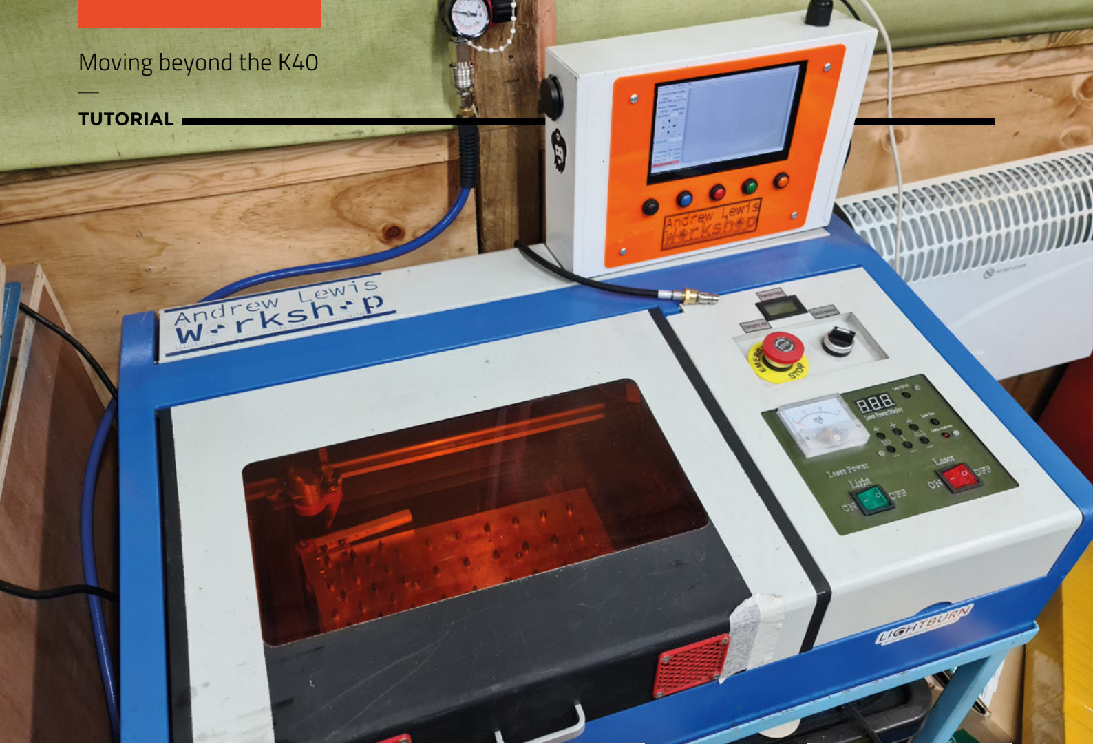
Above ♦ Most images of a K40-type laser look similar, but not the same. That's because most users of the K40 laser modify the machine to suit their own needs. This machine has been modified to add air and smoke assist, laser power monitoring, and has a bolt-on controller added above the laser tube enclosure
