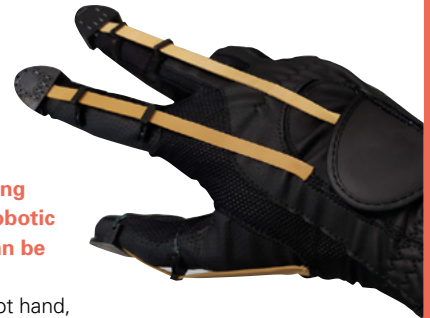
Above ♦ The body-powered exo-glove was designed to enhance the grasping capabilities of the user
