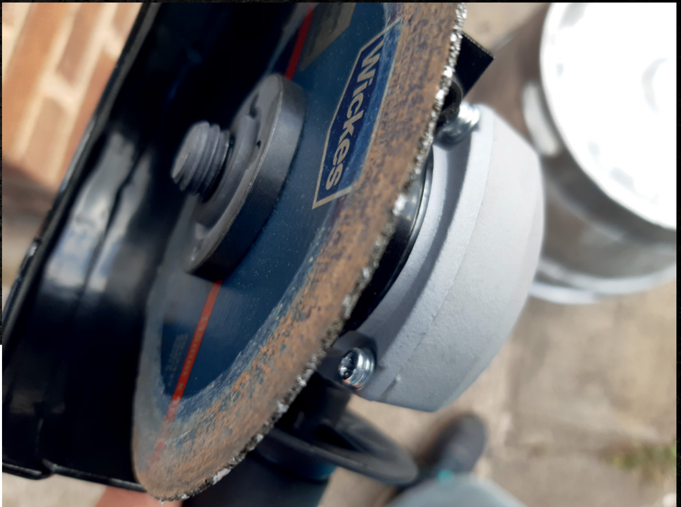
Above ♦ The highlights on the edge of this cutting disc are re-formed aluminium dust. Those bits don't cut anymore; they just get hot
