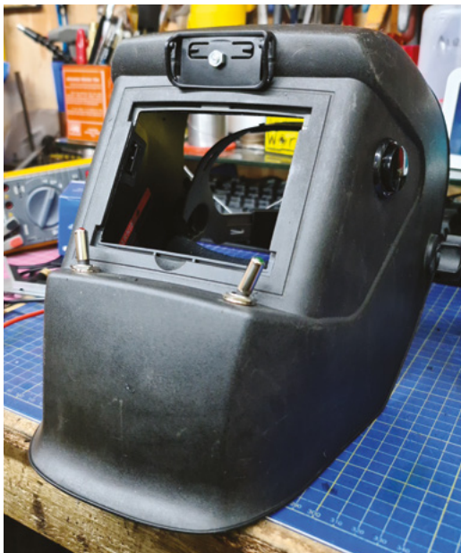
Above ♦ The elastic has been removed from the headlamp bracket, and the bracket has been bolted to the body of the helmet. A rivet, glue, or hook-and-eye fasteners could also be used to fix the headlamp in position
