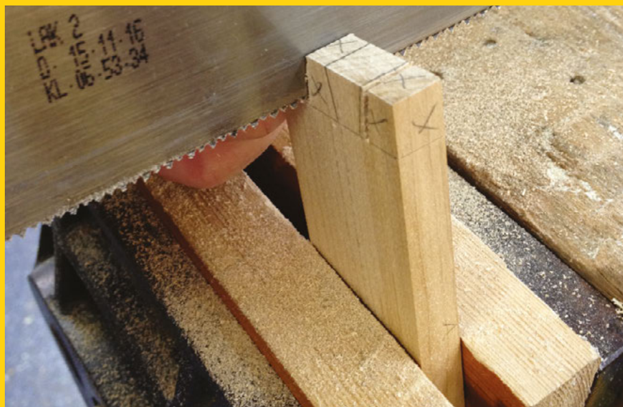
Below ▣ Before you pick up your chisel, saw along the lines you marked
