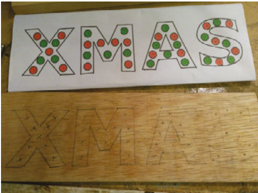
Above ♦ Marking out the backboard
