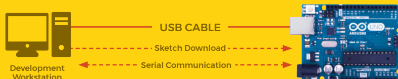
Figure 1 ◆ Arduino development architecture
