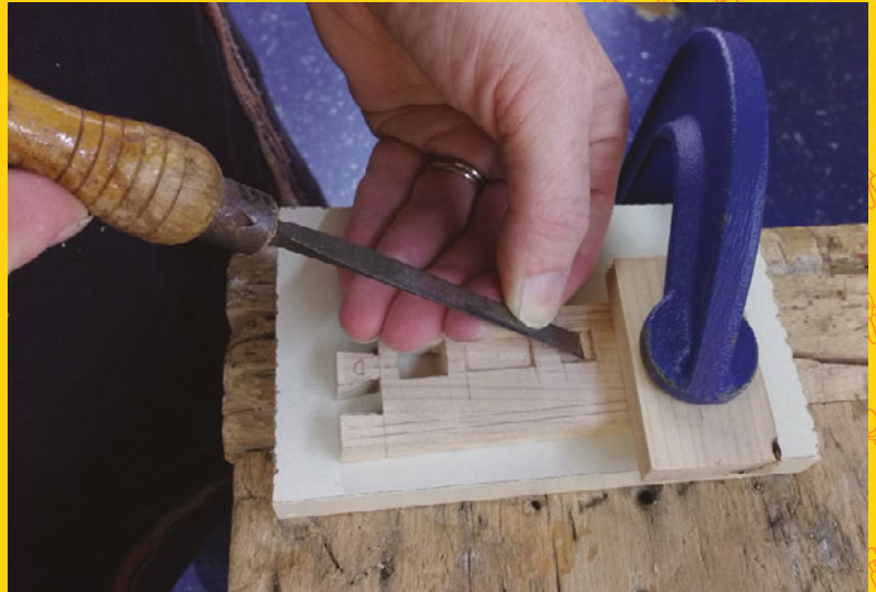
Above ♦ Carving out holes for the Pi's sockets
