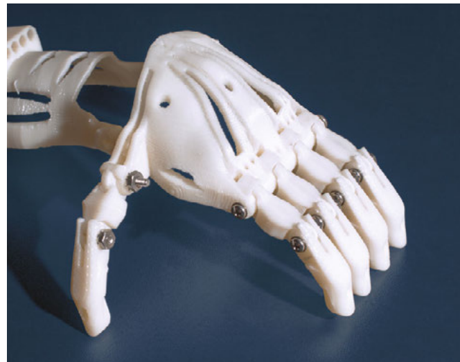
Above ♦ Even the Food and Drug Administration in the US is researching low-cost 3D-printed prosthetics, like this hand that was printed in a Center for Devices and Radiological Health (CDRH) lab
