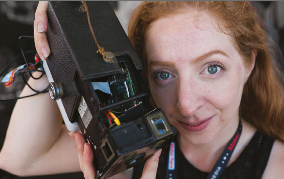
Left You can just see the Raspberry Pi Zero in Becky's smart camera peeking out of the case
