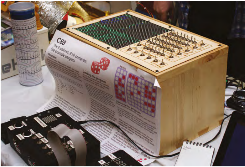
Above Programs are toggled into memory by hand, using tactile switches
