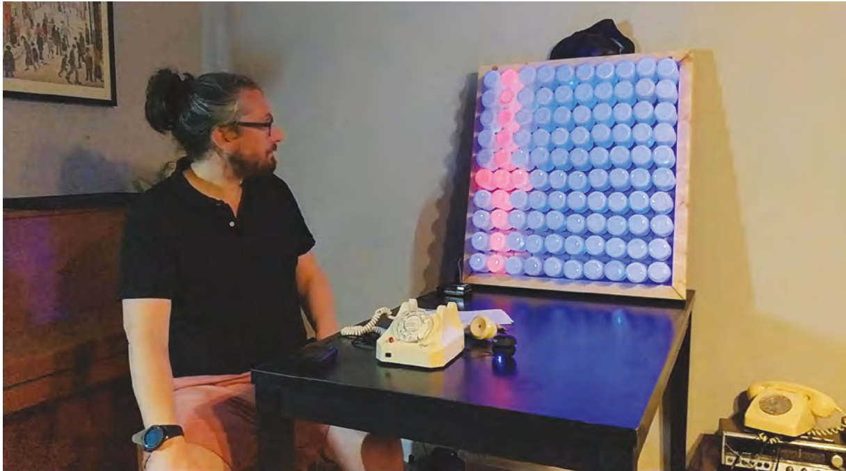
Left ◆ If you're going to do anything with bakelite (which is what the phone case is made from), make sure you take precautions - the old stuff was made with arsenic and asbestos
