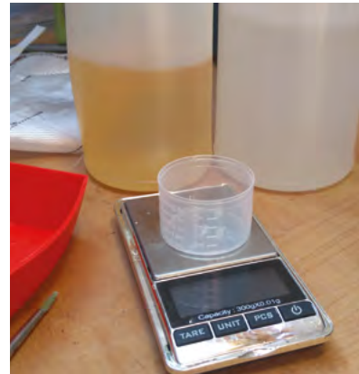
Figure 6 ♦ Using a small set of digital scales to accurately weigh out the correct ratio of resin and hardening agent
