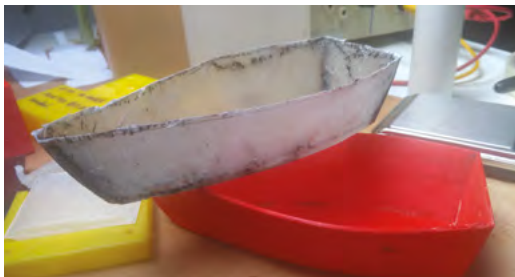
Figure 7 ♦ A freshly 'wetted out' piece of 195g cloth in a small mould. Note the cloth becomes transparent when enough resin is applied
