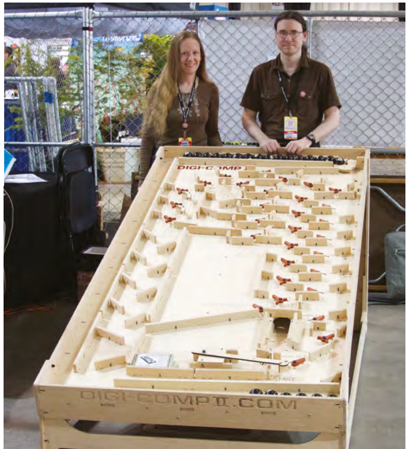
Below ♦ The Digi-Comp II – a gravity powered mechanical computer, seen here in its gigantic form
