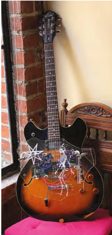
Below ♦ The PCB and electronics suspended above the body of the guitar in version 2
