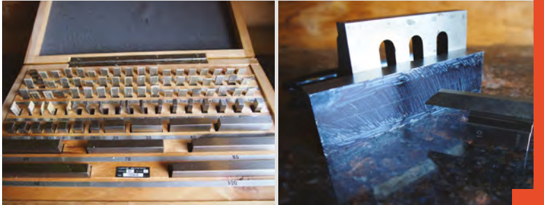
Figure 4 ♦ Scribing the line at 30 mm height onto the stock material using an angle plate to keep the stock vertical
