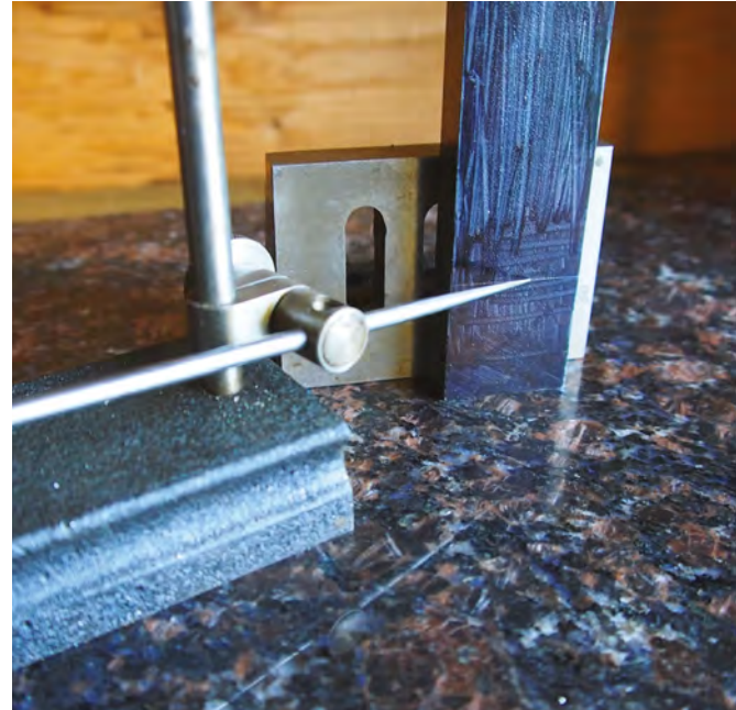
Figure 4 ♦ Scribing the line at 30 mm height onto the stock material using an angle plate to keep the stock vertical
