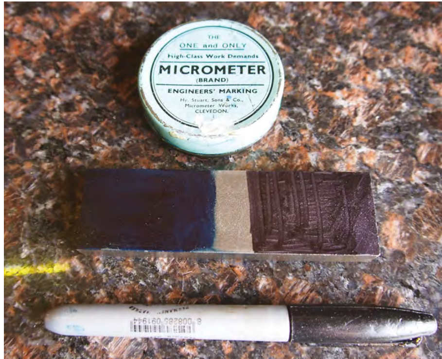
Figure 2 ♦ A tin of engineer's blue versus the cheaper and more available permanent marker
