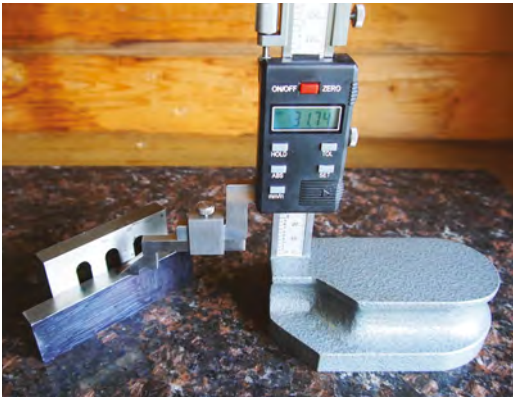
Figure 5 ♦ A height gauge is a versatile tool – it simplifies creating accurate parallel lines at known coordinates on a workpiece, as well as a host of other workshop tasks
