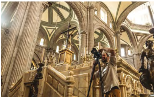
Above ♦ Using 3D laser scanning, photogrammetry, and drones, CyArk digitally captured details of the Mexico City Cathedral
