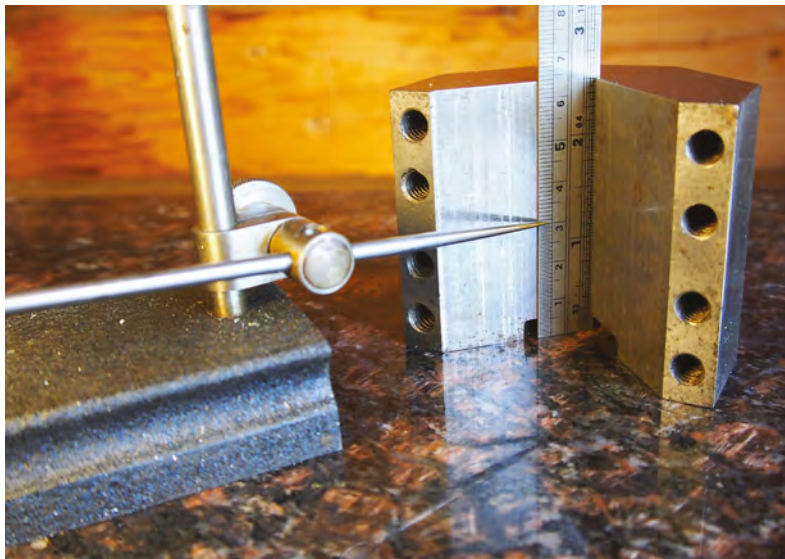
Figure 3 ♦ A scriber held in a scribing block being set to 30 mm height using a ruler held perpendicular to the surface plate with a vee block
